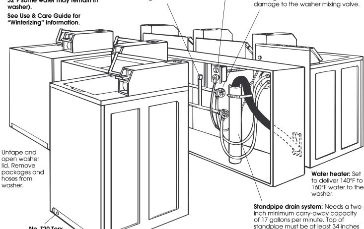
On coin-operated washers, front access to the pump area is available by removing the two, No. 10 Torx screws and then removing the front panel. Non-coin-operated washers do not have a removable front panel. The cabinet and top assembly must be removed by removing clips under console on the non-coin-operated washer.
